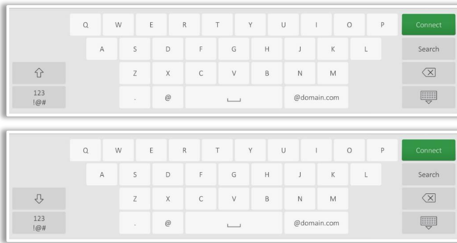
Figure 4 On this keyboard, the shift button changes states, but the letters on the buttons themselves do not.
