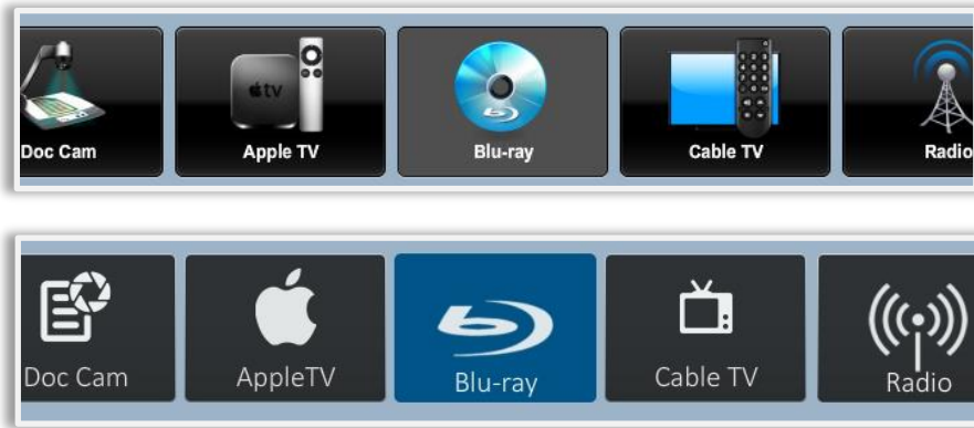
Figure 13 Top: Skeuomorphic icons don't necessarily match real world counterparts, and can take extra time for users to interpret. Bottom: Simplified iconography is more universal, and more easily accommodates a wide variety of active color states.
